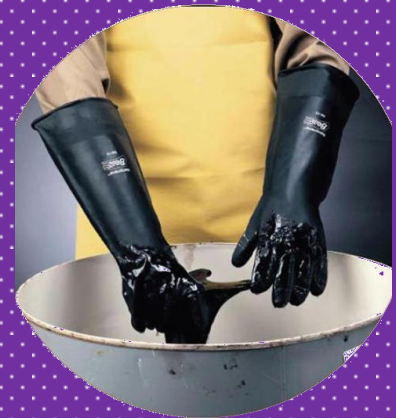
BEST® Chlorofex™ 723, flock-lined Neoprene, 24 mil (0.61mm), 12" (30cm) long; suitable for manufacturing, petrochemicals, laboratories, refining, degreasing, electronic manufacturing.
